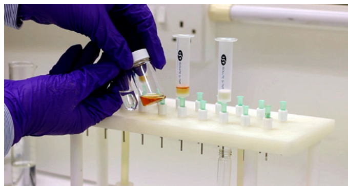
Figure 2d. Comparison, the clear product extract to the left and the original palladium catalyst to the right.
