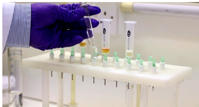
Figure 2c. Metal mitigation complete, the result is a clear product extract.
