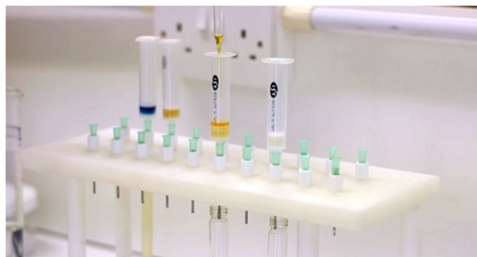
Figure 2a. Crude Pd / mother liquors (500 ppm Palladium) is applied to Si-TMT.
