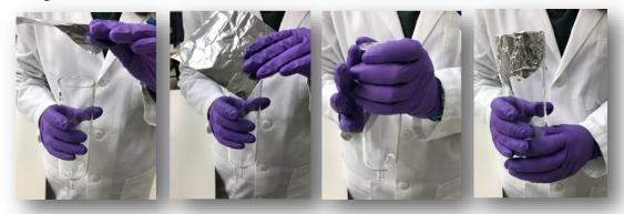
Step 4: Slide the covered evaporation tube into the evaporator, making sure the edges of the tinfoil are trapped along the sides of the tubes.
