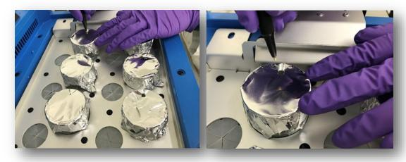
Close the evaporator lid. Visually check the foil over each tube to make sure the nozzle goes through the hole correctly. If a nozzle is resting on top of the foil, twist the tube until the hole in the foil is properly aligned. Then you're ready to start your normal evaporation program!
