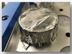
Step 5: Close the evaporator lid and let the nozzles find the top of the aluminum foil. Some of the nozzles will puncture the foil and some will not.
