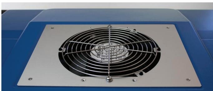
Figure 5. The outlet of the Extrahera top ventilation.
