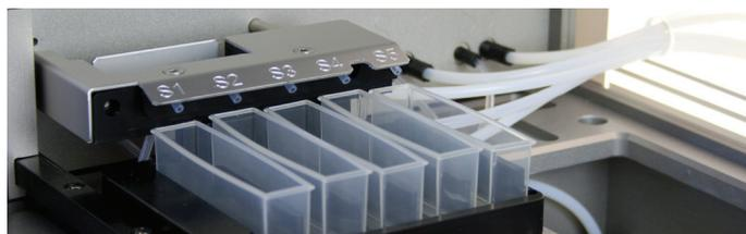
**Figure 56.** The solvent feeder in position to deliver solvent to the five reservoirs in position 5 on the working area.
