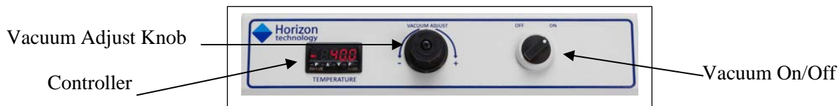
Figure 3-3: Speed-Vap IV Controls
