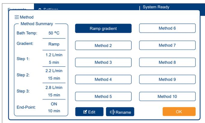
**Figure 29.** The Method view where you select the method you want to run, or modify a method and then run it.
