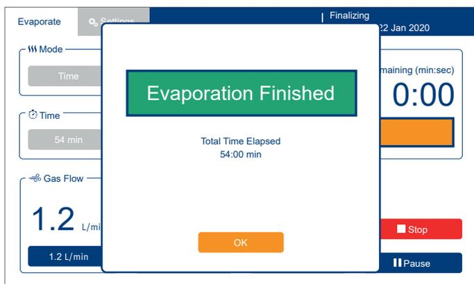
**Figure 27.** The Evaporation Finished dialog is displayed when the specified evaporation time is reached or the end-point level (+ any additional time) is reached for all tubes.
