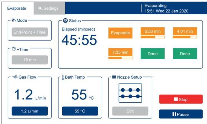
Figure 24. The Evaporate view when end-point + time mode is selected.
