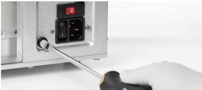
Figure 37. Removing the fuse holder.
