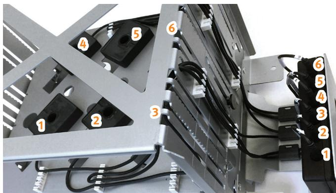
Figure 36. The wiring of the end-point sensors.
