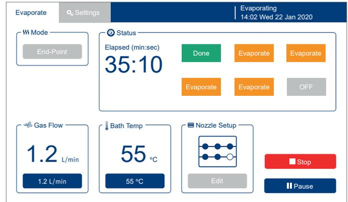
Figure 25. The Evaporate view showing one tube that has reached the end-point level.
