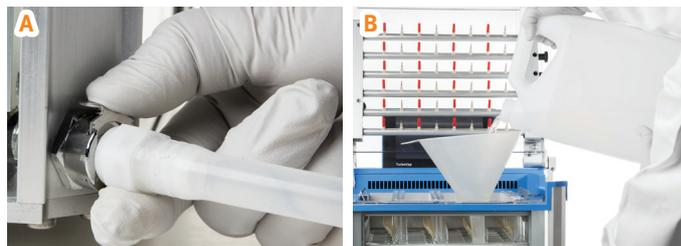
**Figure 18.** A: Disconnecting the drain tube by pressing on the top of the DRAIN port. B: Add deionized water until the water's surface is as high as the initial liquid level will be in the tubes but not higher than just below the blue water bath top cover.
