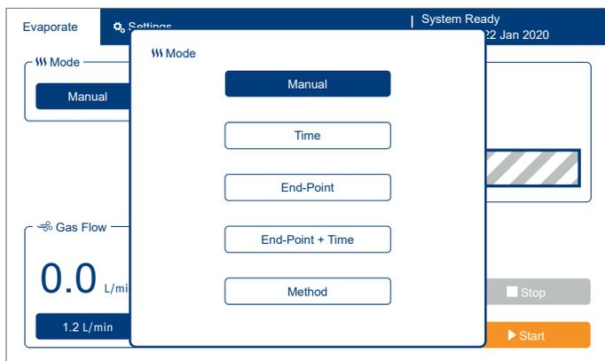
Figure 22. The different evaporation modes that can be selected.
