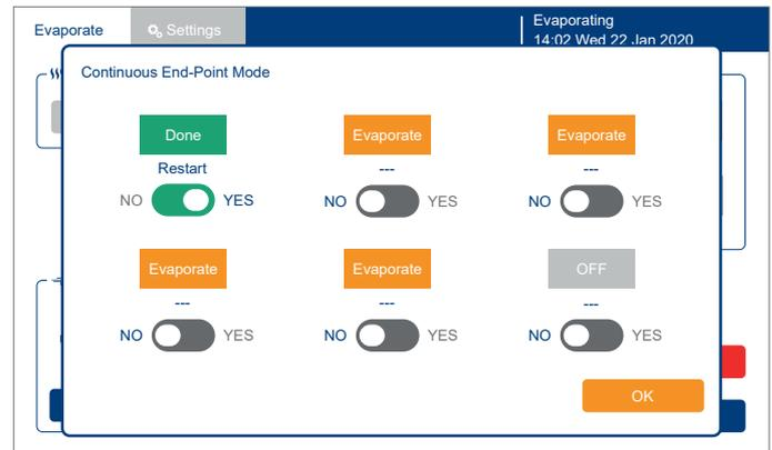
Figure 26. The Continuous End-Point Mode dialog showing one rack position that can be restarted.
