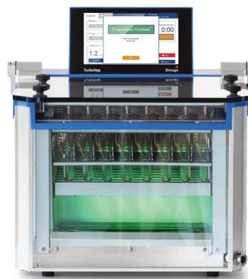
**Figure 11.** When a run is completed, the light in the water bath changes to green.
