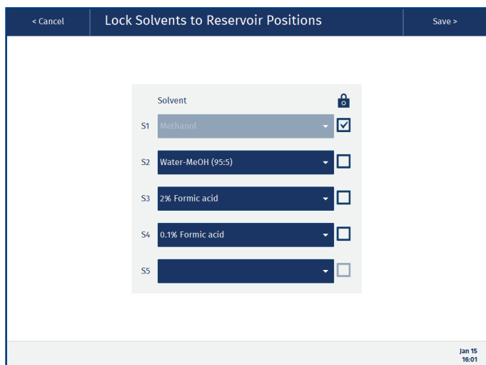
Figure 2. The Lock Solvents to Reservoir Positions view with methanol locked to reservoir S1.
