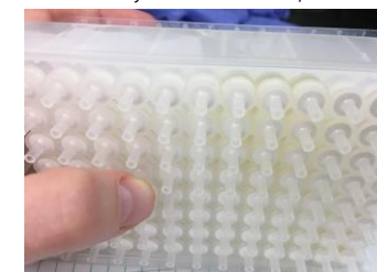
Figure 5: EVOLUTE® HYDRO CX plate after hydrolysis incubation showing that sample is held above the sorbent for the duration of hydrolysis
