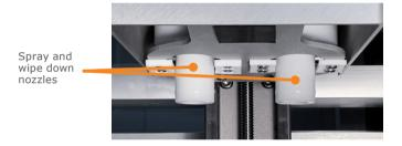
Wet a lin-free paper towel or kimwipe with 70% – 80% alcohol spray and wipe the ejector and ejector pads.
