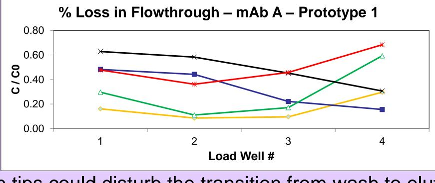
Residual liquid in tips could disturb the transition from wash to elution, resulting in low recoveries
