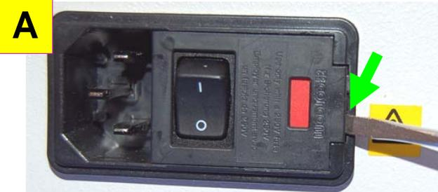
Remove the power cord from the power mains. Use a small screw driver to open the panel (A).
