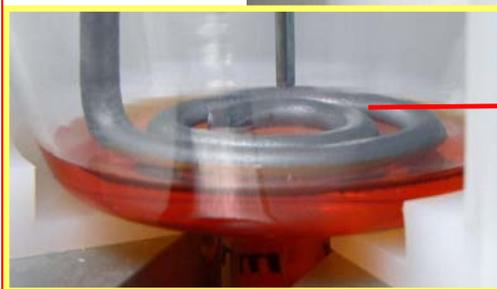
If after pressing the Start button, the heater turns off and the heating element is partially exposed as shown here, repeat the process again and press Start a little bit earlier.
