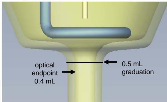
Select this tube when the objective is to add volume such as an internal standard to bring to 0.5 mL volume.
