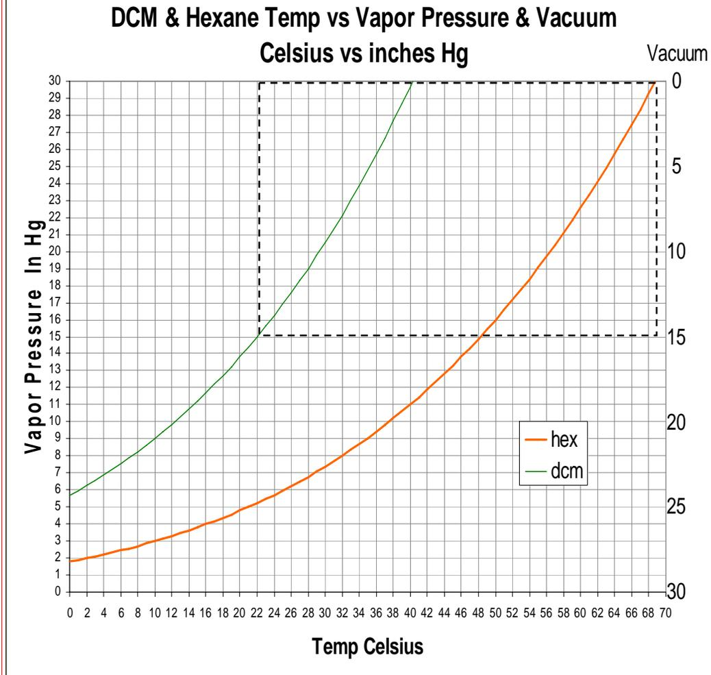
**Notice:** If the temperature indicates a lower vacuum, turn off the sparge gas and re-run the test. The addition of sparge gas into the concentrator tube will reduce the overall vacuum level.
