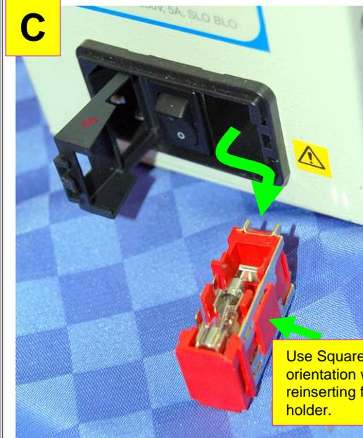
Use Square for orientation when reinserting fuse holder.
