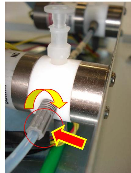
3. Finger Tighten Each Bottom Compression Screw (nitrogen feed line). The nitrogen feed line is black polyurethane tubing. Turn fitting counter-clockwise when viewing valve from top.
