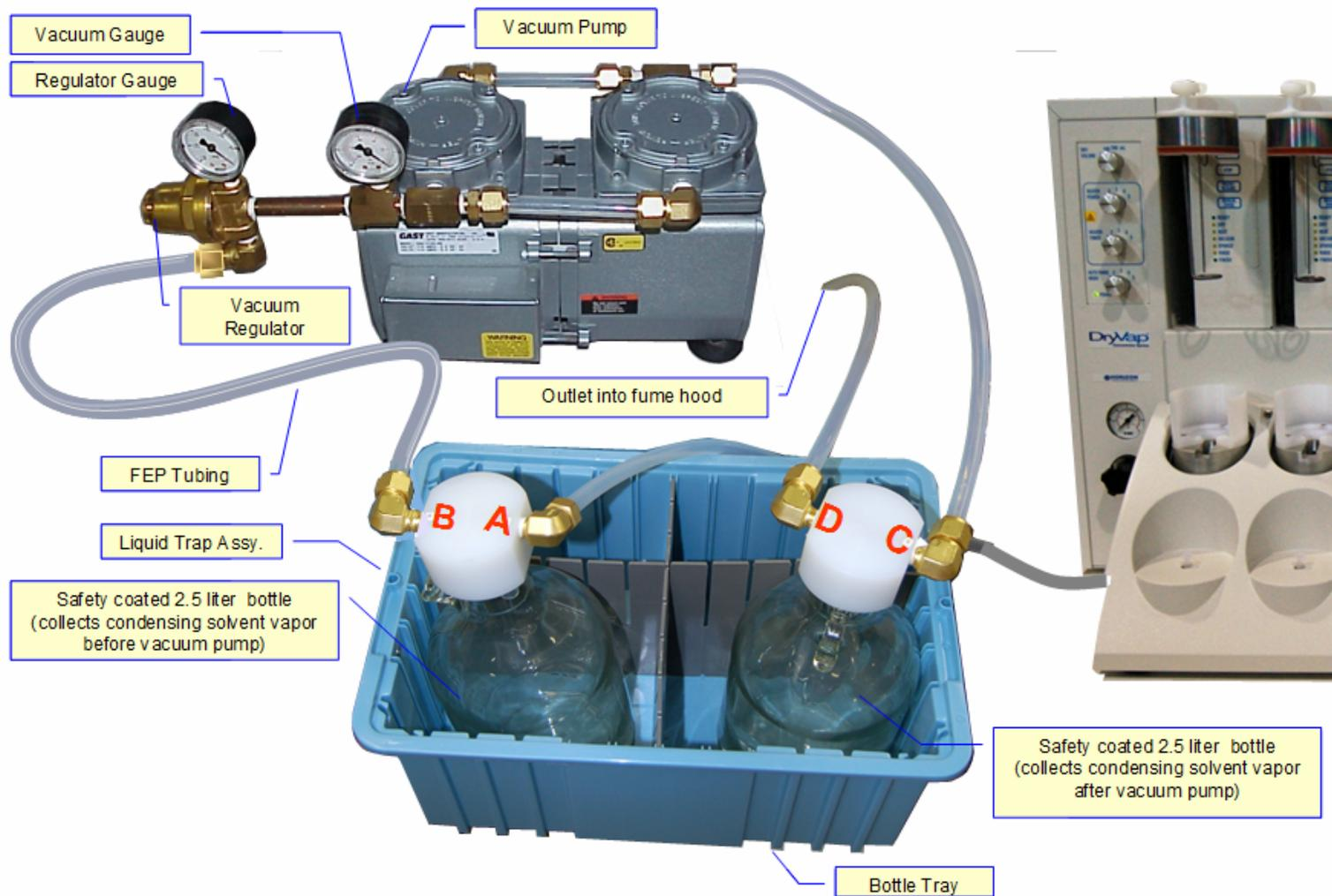
Figure 3-3: Liquid Trap Assembly
