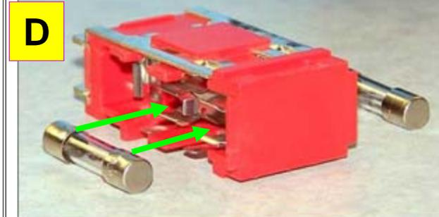
Replace fuses on both sides of holder. Use the two adjacent clips for these short fuses.
