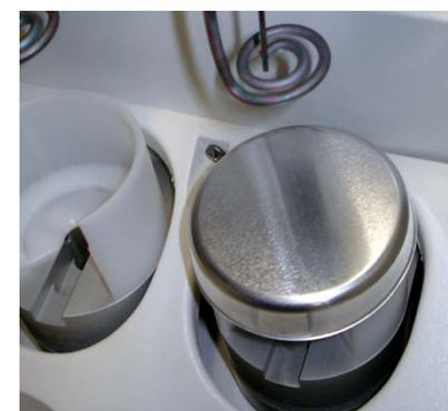
Cover the cradle when cleaning heaters, to keep the sensors and the tube flag in optimal condition.
