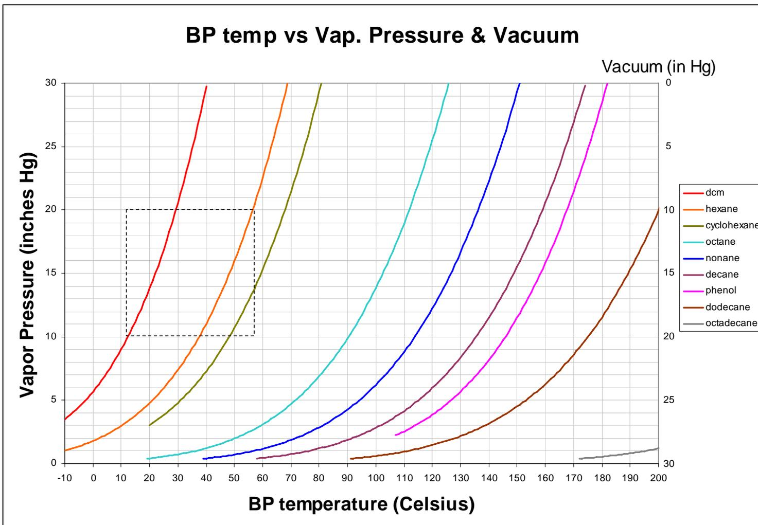
DCM and Hexane are common solvents used for sample extractions. The dotted line box indicates the BP range of the two solvents between 10 and 20 inches of Hg vacuum. Increasing the vacuum decreases the vapor pressure on all solvents and analytes. Vacuum exceeding 20 inches Hg show the beginning of convergence of the vapor pressures and BPs.
