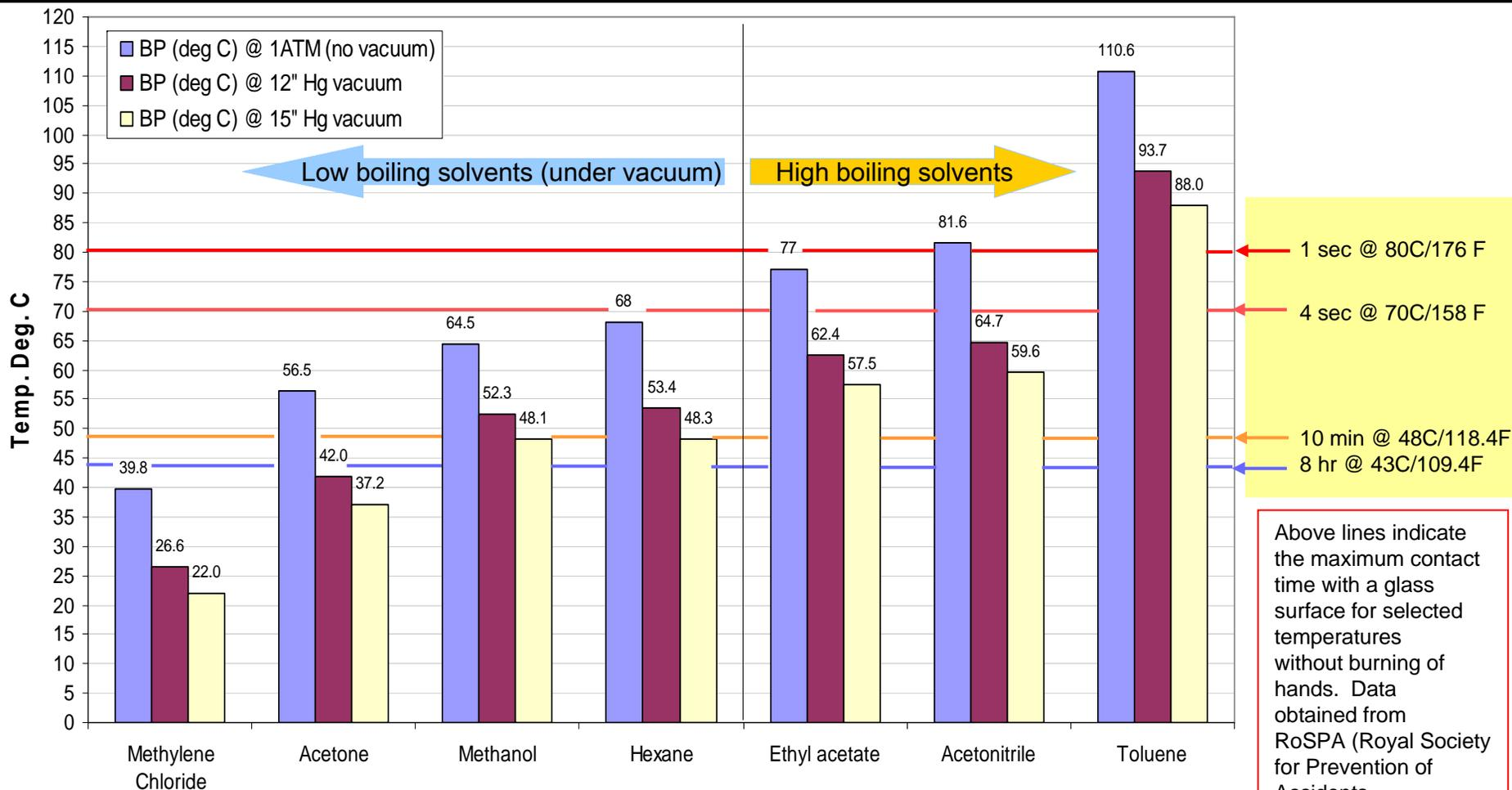
BP for solvents under 12 and 15 inches Hg vacuum were calculated using the Antoine Vapor-Pressure equation and Table 5.9 (Vapor pressures of various organic compounds) p5.39 Lange's Handbook of Chemistry 14<sup>th</sup> ed.
