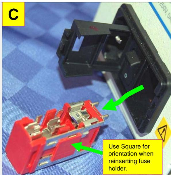
Pull the fuse holder out. Note the square on the fuse holder must be on this side when reinserting holder back into power mains. It will not fit in the reverse orientation.
