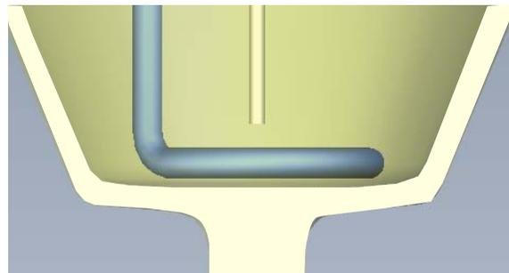
Select this tube when the objective is to totally remove solvent from the sample or for evaporating the sample to volumes > 1 mL (no optical endpoint).
