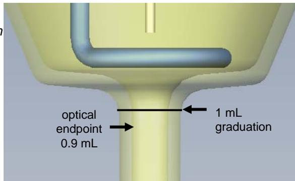
Select this tube when the objective is to add volume such as an internal standard to bring to 1 mL volume.
