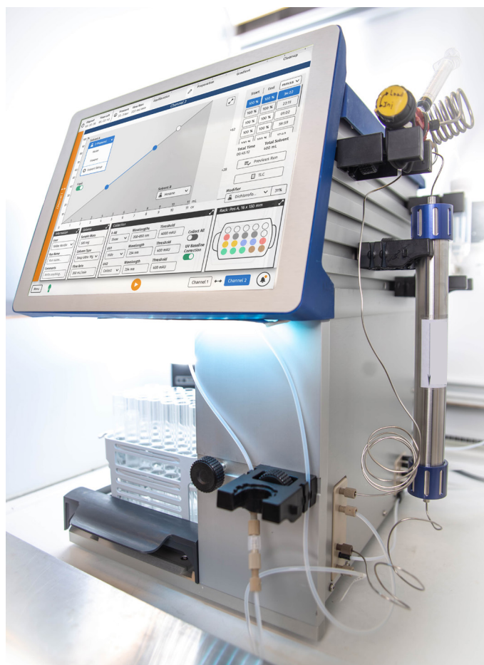
Figure 2. The semi-preparative HPLC column setup on Biotage® Selekt.
