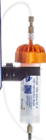
Biotage Selekt Enkel has one channel and column attachment on the side only.
