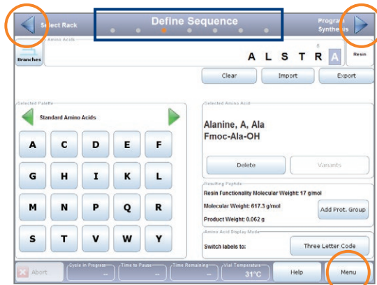
The peptide sequence is defined in the third step of the synthesis wizard.
