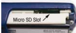
Figure 4A: Micro SD slot
