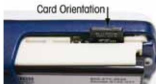
Figure 4B: Micro SD card in slot
