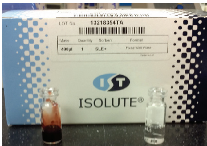
Figure 2. Fortified whole blood sample and subsequent extracted cannabinoids in MTBE prior to dry down.
