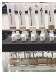
Figure 1. Initial Colorimetric Screen using 500 ppm Grubbs catalyst solution in DCM, (left to right: ISOLUTE® Si-Thiol, ISOLUTE® SCX-2, ISOLUTE® Si-Trisamine, ISOLUTE® Si-TMT and Biotage® MP-TMT).
