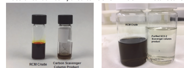
Figure 6. a) left crude reaction passed through activated carbon b) right - crude reaction passed through ISOLUTE® SCX-2 metal scavenger.
